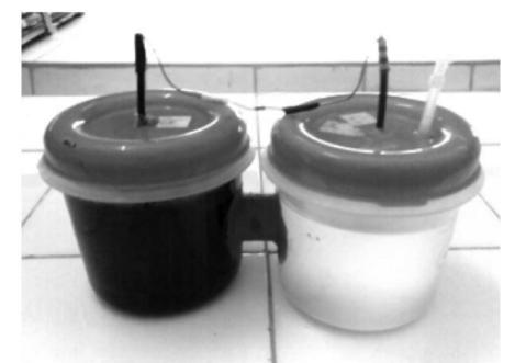
Arboleda constructed several of these makeshift MFCs using simple materials to test the power generation potential of several substrates
